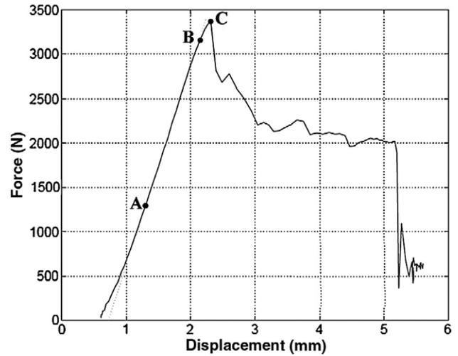
**Fig. 2.** Representative force-displacement graph. The y-axis is force (in Newton, N) and the x-axis is displacement (in mm). Femoral strength (i.e., failure load) was taken as the maximum force sustained (point C), and stiffness was defined as the slope of the linear region (segment AB).
