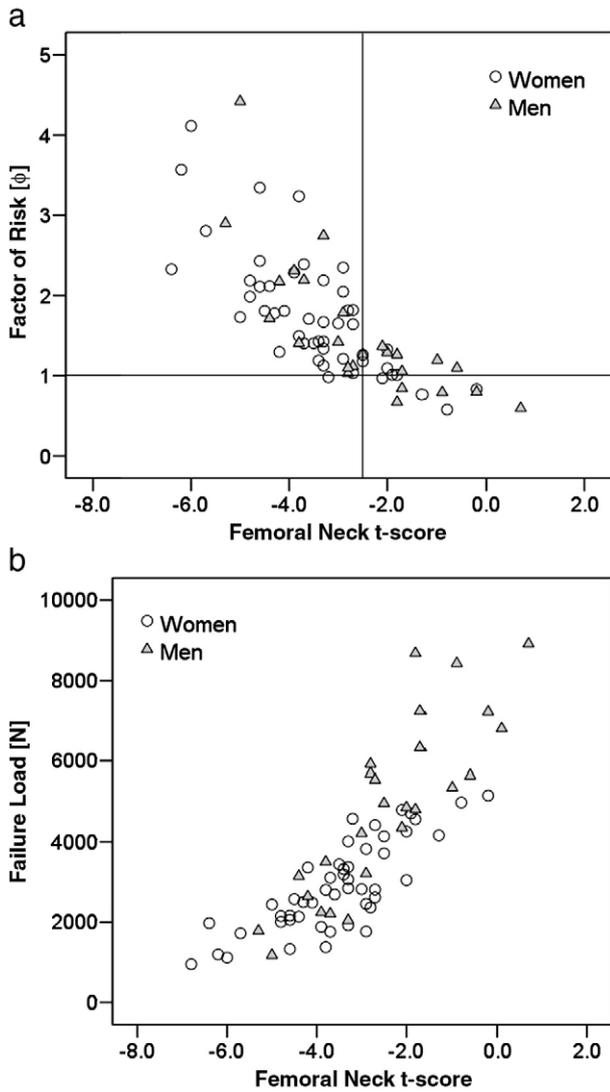
**Fig. 4.** Factor of risk for hip fracture ( $\phi_{\text{atten}}$ ) vs. femoral neck BMD T-score and failure load vs. femoral neck BMD T-score. Lines are drawn on the graph at femoral neck T-score = -2.5, and at  $\phi_{\text{atten}} = 1$ . The regression equation for FN aBMD vs.  $\phi$  is  $y = 0.687e^{-0.253x}$ .
